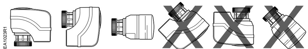
**Figure 5. Mounting Position.**
