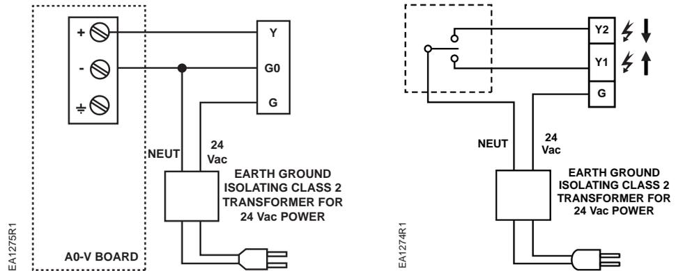
Figure 6. SSA/P61U Wiring Diagram. Figure 7. SSA81U Wiring Diagram.
